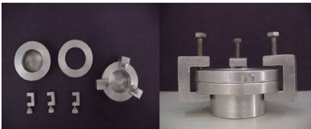
Fig. 4. System adapted from Payne's permeability cups (Braive Instruments, Liège, Belgium), according to 'B' method of ASTM guidelines E96-66.
